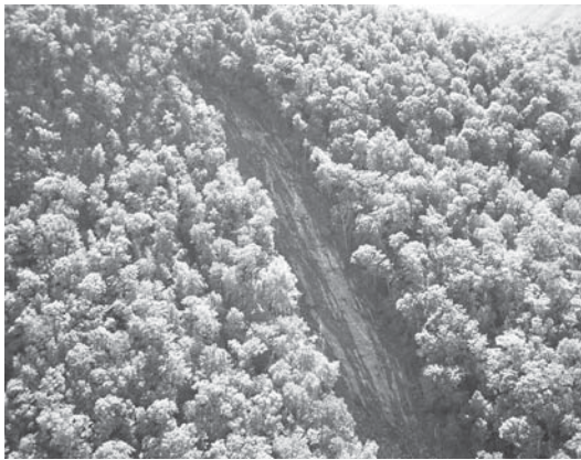
Figure 11: The head scarp of the Peeks Creek flow near the crest of Fishhawk Mountain. The overlying soil was ripped away, exposing the underlying bedrock for several hundred meters down the channel of the flow (courtesy of the North Carolina Geological Survey).
